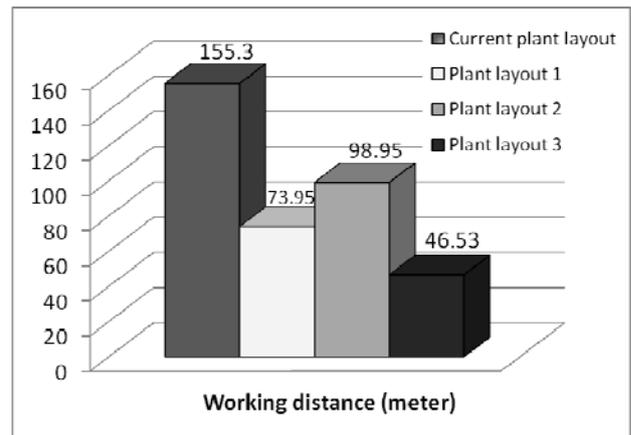
Fig. 4 Reduction in working distance with improved plant layout designs.
