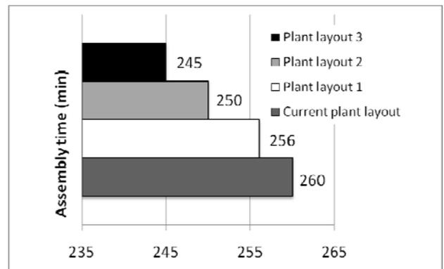
Fig. 5 Improvement in average time of operation with improved plant layout designs.
