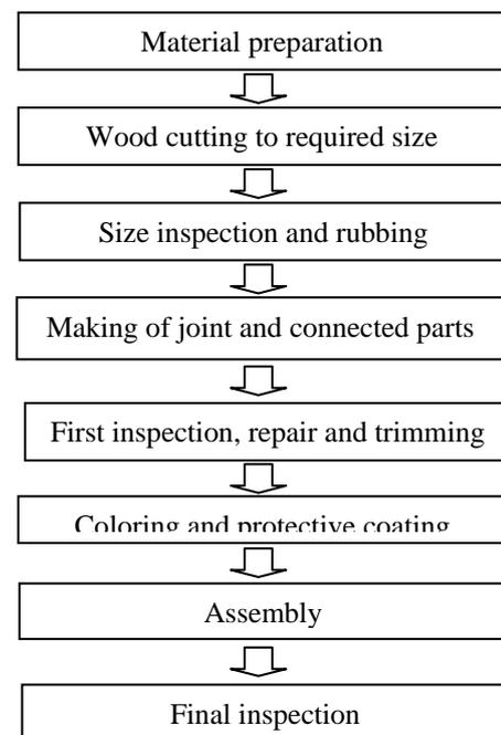
Fig.1 Typical process diagram of a wood table.
