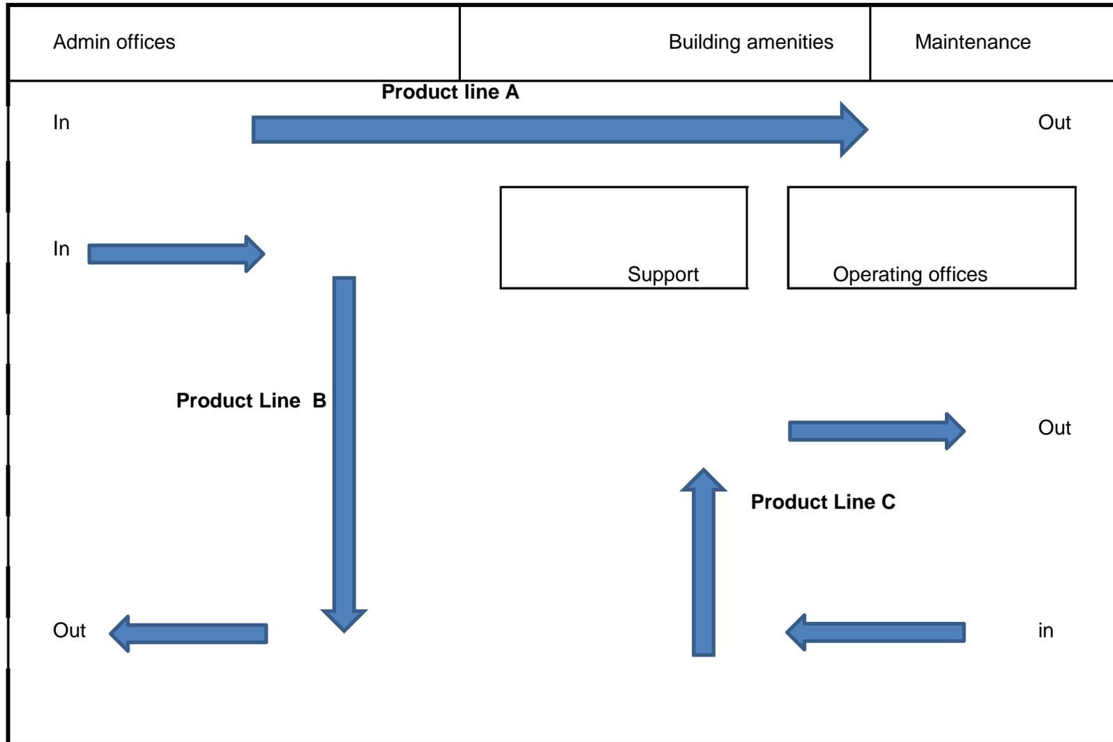
**A 4 To place permanent equipment and avoid later interference**
