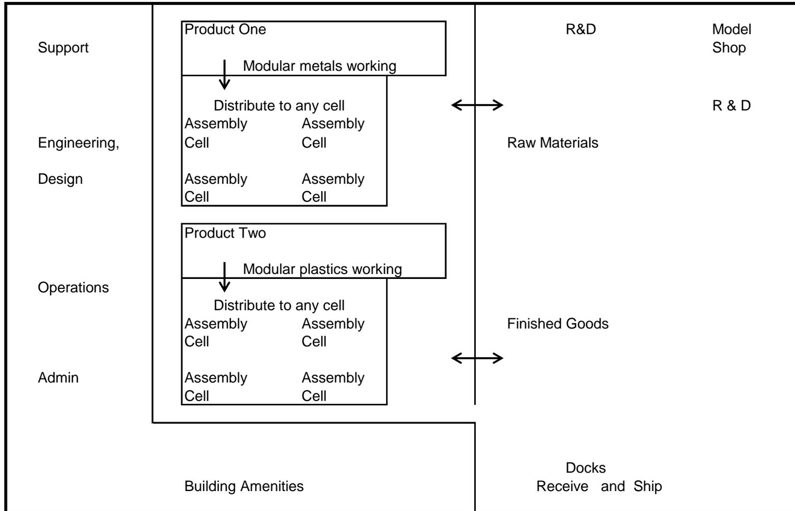
**A 13 Electronics fab and test**
